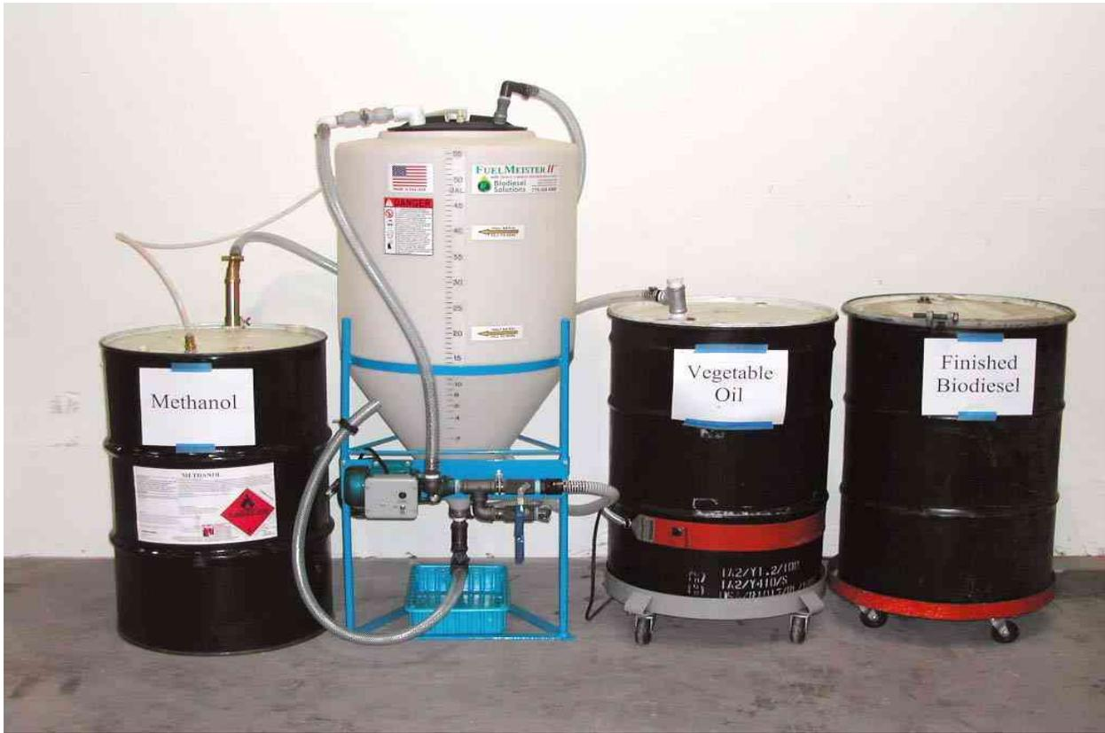
Typical set up for single tank system and user supplied drums.
