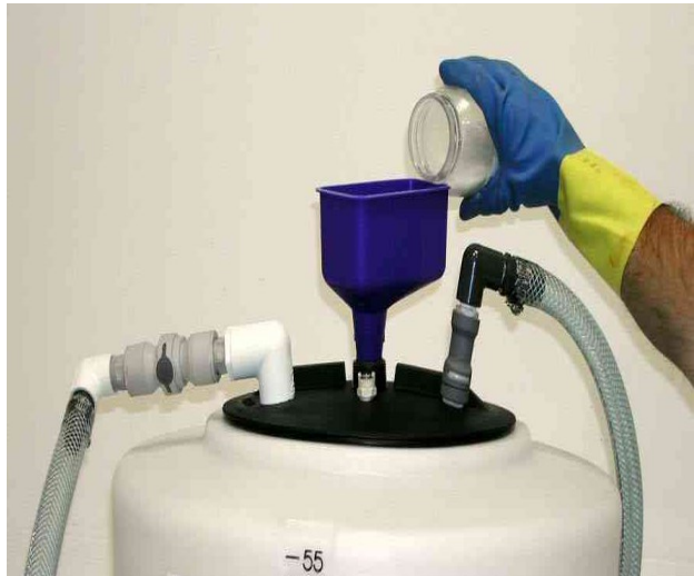
Adding lye into the catalyst injection lid.
