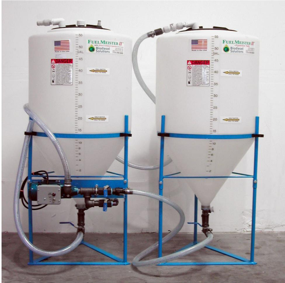
Dual tank system with separate wash tank.
