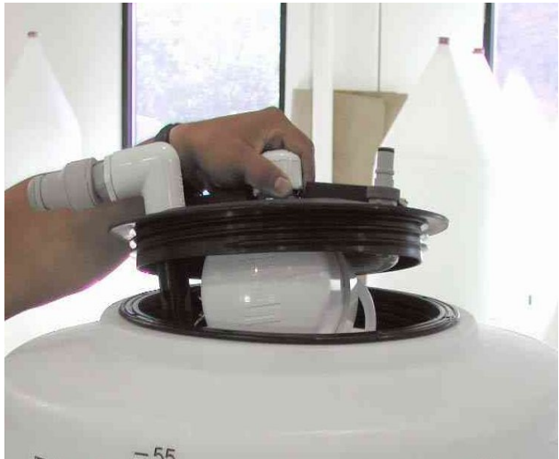
Catalyst injection lid showing venturi real time mixing chamber on bottom side.
